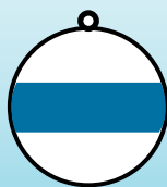
MOORING BUOY White with reflectorized blue band. May have white light or reflector.
